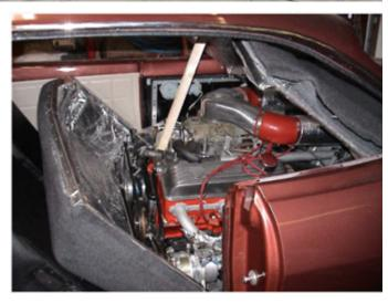
*Electric Rear Windows.* It would be awfully tough to retain the original hand-operated window cranks for the rear quarter windows with the mid-mounted engine and headers in the way. The rear quarter glass is motorized by coupling window drive motors from a Camaro to the Corvair window crankshafts with a custom built coupler. The window crankshaft is drilled and the coupler is connected to the shaft with a pin. The coupler mates with the gear on the window drive motor – simple and effective.
