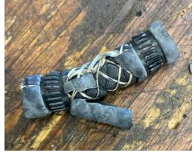
layers eventually disintegrate. Dayco does make submergible fuel hose; check Summit Racing as well as better auto parts stores such as NAPA.
