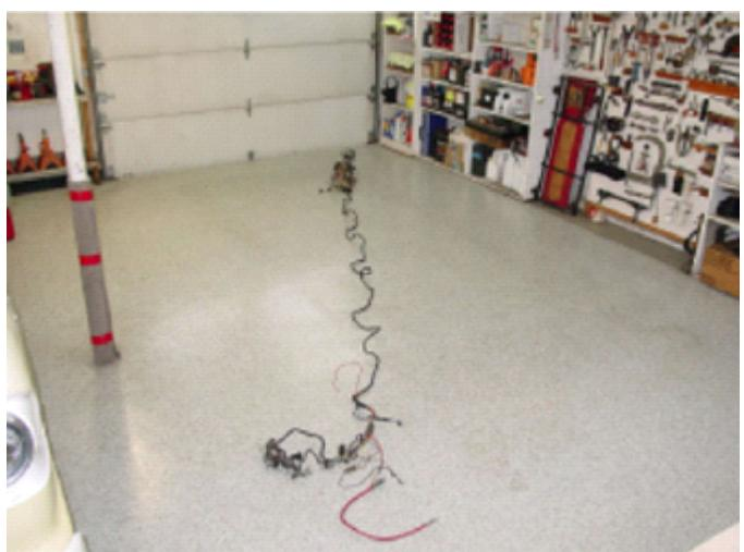
battery post, travels to the ignition switch, turns around and travels back to the starter solenoid. An easily understood routing - however, during that routing the current has to pass through 10 push on connections, 2 switches and 15 crimp connections. There is only one soldered connection in the entire starting circuit.
