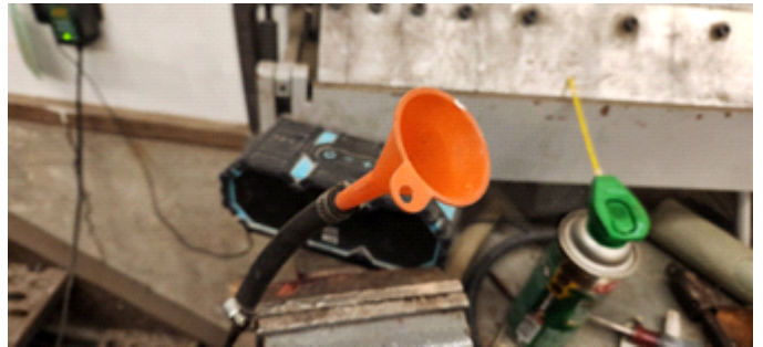
Simple funnel attached to hose for gravity lube.
