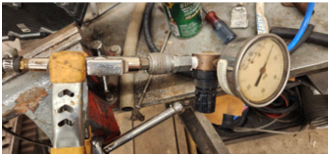
Compressor air-hose to fuel-hose adapter.
