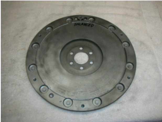
Stick-shift Corvairs have an unusual 2-piece flywheel that was hot-riveted from the factory.
