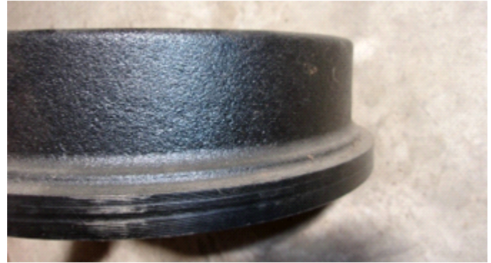
The brake drum width for late model Corvairs is 2.0 inches for the front (above) and 2.5 inches for the rear (below). Don't mix 'em up!
