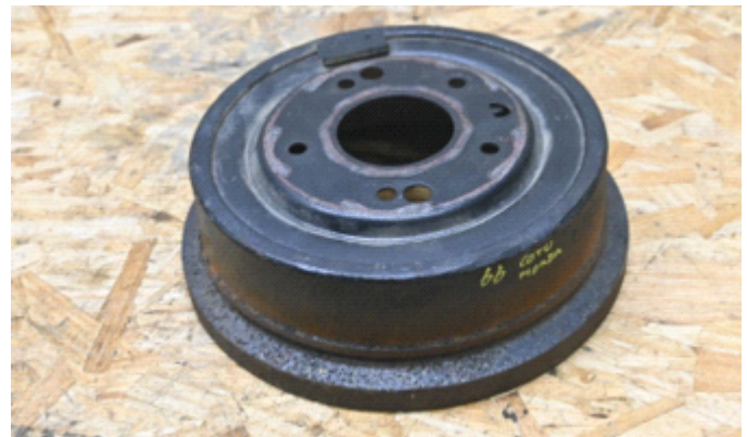
The brake drum width for late model Corvairs is 2.0 inches for the front (above) and 2.5 inches for the rear (below). Don't mix 'em up!
