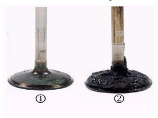
(1) Intake valve: 10,000 miles with TOP TIER Detergent Gasoline
