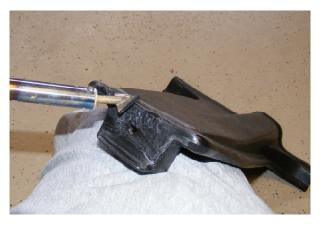
I then just moved the "iron" around the plastic, melting and molding the two pieces together.
