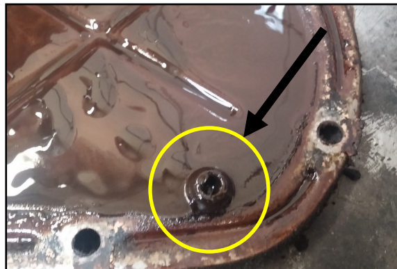
Differential cover with plugged vent hole at bottom right corner
