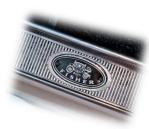
The sill plates are soft material and scratch and dent easily. Knock your shoes together outside the car before swinging your legs under the dash.
