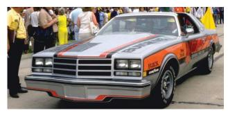
**7. 1976 Buich Century Indianapolis 500 Pace Car** Buick's turbocharging legacy was established with this purposeful pace car. Engineers leveraged the recently revived, more-efficient 3.8L (231 cubic inches) V-6 engine that was supplanting larger V-8 engines in many production models. They filled it with 22 psi of turbo-fed boost - resulting in 306 horsepower from the compact powerhouse - and reset expectations for Buick performance.
