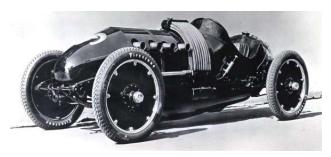
2. The 1910 60 Special, or "Bug," was built by the Buick racing team and had a unique nosecone - a feature designed more for aesthetics than aerodynamics. A huge, 10.2L (622 cubic inches) four-cylinder engine propelled the Bug to 110 mph. Buick built two 60 Special racecars, one for Prest-O-Lite Trophy winner Bob Burman, and a second for another racer of note: Louis Chevrolet.
