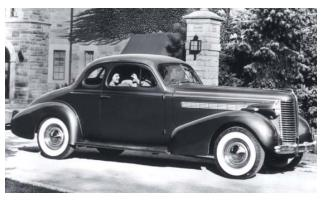
**3. 1938 Buick Century** Buick introduced straight-eight engines in 1931, but it was the 1938 Century model that established a new performance benchmark. Dubbed Dynaflash 8, the 5.2L (320 cubic inches) inline engine featured new, domed pistons that contributed to an 11-hp increase over the 1937 engine. It was enough power to pass the "century mark" at 103 mph, making the Century one of the fastest cars of its day.
