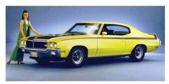
**6. 1970 Buick GSX** At the height of the muscle car wars, torque was king and no competitor could dethrone the 510 lb.-ft. (678 Nm) of twist generated by the GSX's available 455 Stage I V-8 engine. In a 1970 road test, Motor Trend went from from 0 to 60 mph in 5.5 seconds and covered the quarter-mile in 13.4 seconds. The GSX's combination of raw power and Buick's signature luxury prompted many to describe the car as a "velvet hammer."
