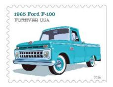
> The 1965 Ford F-100 that had a new grille featuring 18 small rectangular openings. It also featured what Ford dubbed a "Twin-I-Beam" independent front suspension.
