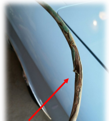
Cable housing showing the exterior, cracked and broken. The inside is rusty. This piece was near the rear wheel well.
