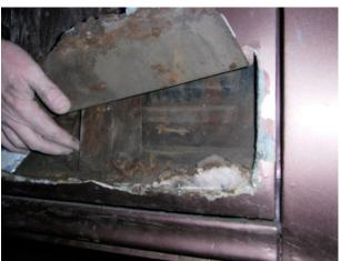
catastrophic outcome. We got all the bolts out, cleanly, that were screwed into the ramp. First we cut off the end of the bolt that was outside of the nut – so we wouldn't have to screw all that bad thread through the nut – then the old "smoke wrench" was applied to 'cherry' up the nuts. The nuts are welded to the ramp so they will remain while the heating releases the trapped in bolt.
