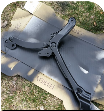
Replacement section, primed, painted, and ready to be installed.
