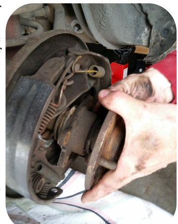
After the axle bearing retaining bolts are removed, the axle just slides out of the brake backing plate.
