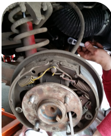
Removing the axle bearing retaining nuts and U-Joint bolts to release the axle
