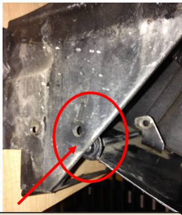
FIGURE 1: Note the hinge pin was installed backwards, and now has no way to be retained in the hole.
