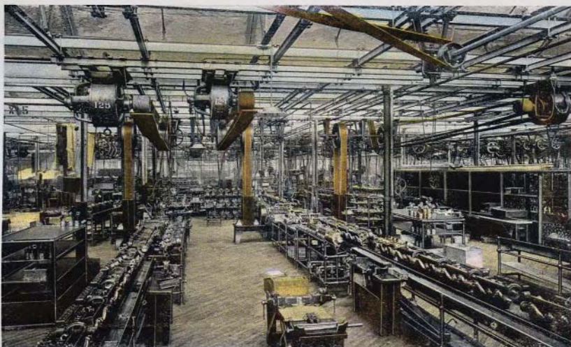
MOVING CONVEYORS HASTEN THE MOTOR ASSEMBLY.
