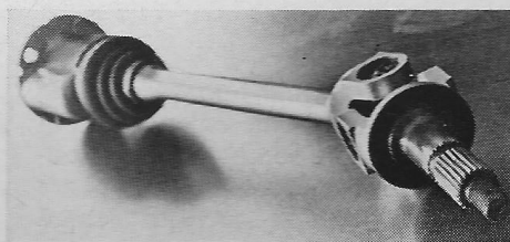
The forged, polished-all-over U-jointed Cardinal axle shaft.
