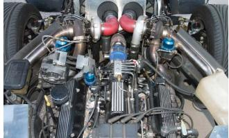
wanted 25 MPG and planned to drive the car until the wheels fall off, so the turbos can't be overly large or too race-prepped. I found a pair of Schwitzer turbos that were John Deere tractor spec, and sent them up to London Ohio, along with a pair of stainless steel racing waste gates for the fab work.
