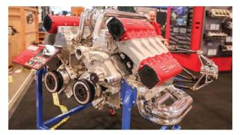
This is a twin LS V-8 setup intended for a Hal Design supercar. It features two separate 427 cubic-inch engines linked together to power a single transaxle. There may be easier ways to get 1400 horsepower, but not many of them would look this cool.
