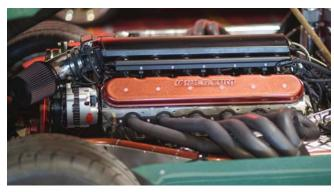
This Cheetah is powered by an iron-block V-12 from the Australian company Racecast. The V-12 is based on Chevrolet LS architecture and is available in 564- or 580-cubic-inch versions. They weigh 584 pounds in cast iron form, and produce 700–1000 horsepower.
