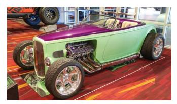
Jordan Quintal at Super Rides by Jordan built this Boyd roadster more than a decade ago, and it was back at SEMA as a tribute to the owner, Steve Barton. The monster V-8 engine uses 4.9-inch bores and a 6-inch stroke to deliver 904 cubic inches. It has dual overhead cams with four valves per cylinder. Even in its "detuned" street trim it produces 1500 horsepower.
