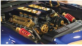
The Roadster Shop's widebody second-gen Camaro, Road Rage, has a lot going on under the hood. While a cantilever suspension puts the coilovers on display, it's the LS engine that steals the show. Its individual throttle bodies are fitted to squared-off bell mouths that protrude through the hood and mimic 1969 Camaro hood louvers.
