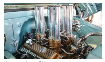
This gen-one Chevy small-block is hiding its electronic injectors in the valley, giving the illusion of mechanical fuel injection.
