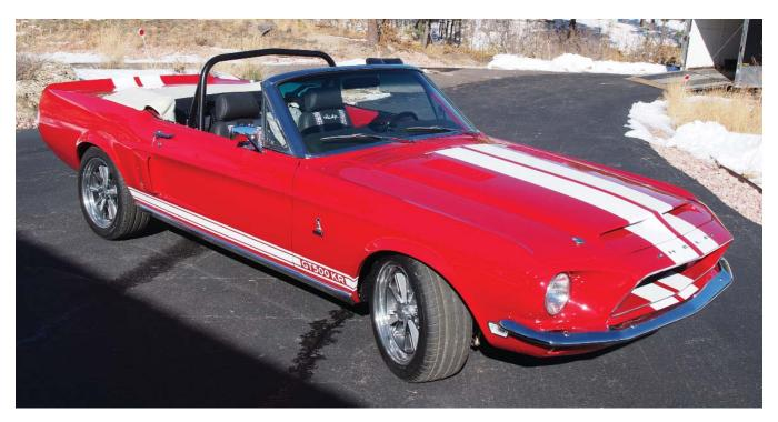
This is story about my 1968 Mustang Shelby GT500KR Convertible Tribute car. This was a 2 year custom build project starting with a somewhat rusted out 6 banger car from San Diego, CA. The only original parts used were the 4 corner panels, the 2 doors, the front windshield frame, the dash and the back seat. All other parts were custom or OEM parts.
