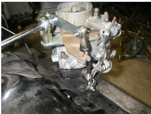
110 or Two Carb Linkage Kit used with manual choke
