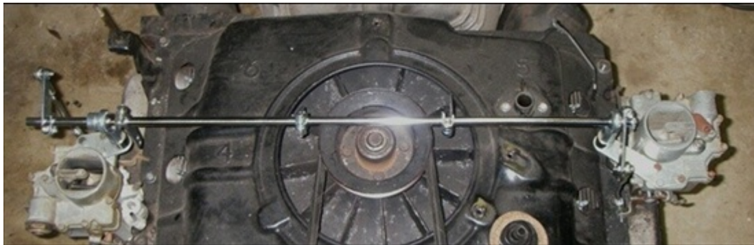
Linkage Kit for 1960 (Motor is 1964)
