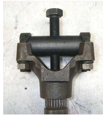
Yoke Puller installed for use on 1960-64 Axle
