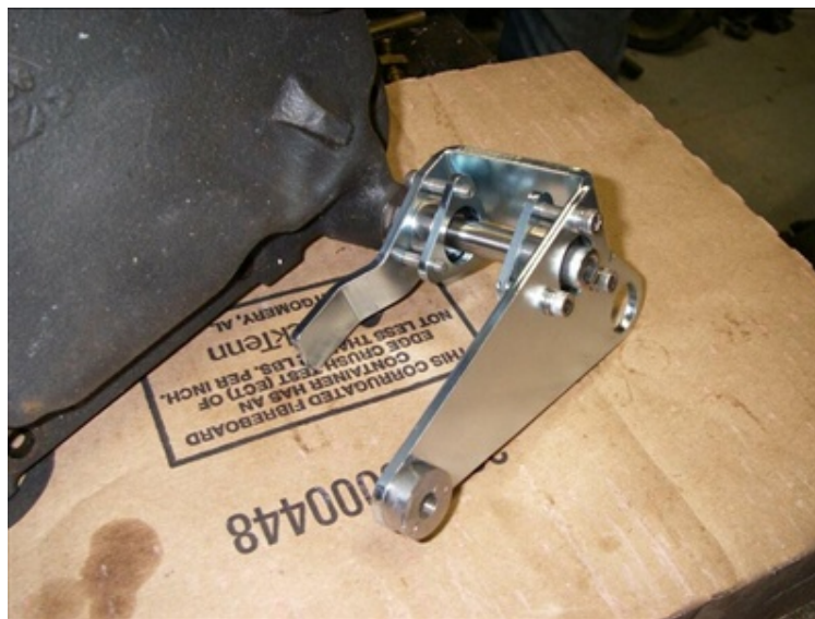
1966-69 3sp & 4sp Manual Transmission Pivot Shown with 5/16 Bolt. Also available with 3/8" Bolt.
