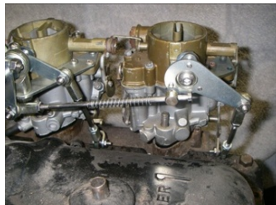
1966-69 140hp Right Side. Using Choke Lock-Outs.
