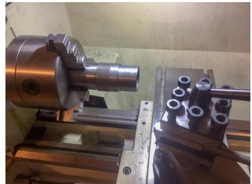
Step 3: Turn down the OD of the sleeve material (I chose chromoly tubing with a .188 wall thickness) so it is just a little bit larger than the ID cut in the carrier halves to make a good press fit. (Right)
