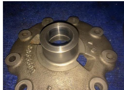
Step 5: Bore the ID to get a nice fit to the axel yokes (about .002 over), and trim off any excess sleeve material. (Right)
