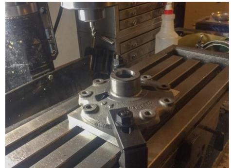
Step 2: We first need to bore out the ID the carrier halves to allow the insertion of a steel sleeve. What turned out to be the biggest hassle, was to get the part centered in my 4 jaw chuck! (Left)
