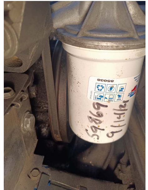
Above; Note pulley rubbing filter.
