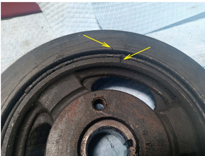
Notice outer ring pulled away from center and mis-alignment of the hash marks. This balancer is a goner...
