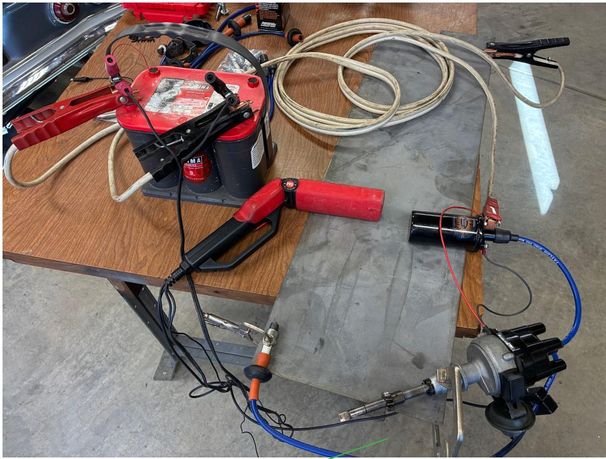
*Even a Minimus Edition gets some pix! For those of you who've survived the Editor's whining about not being able to start up the Yenko Stinger, this is the test fixture cobbled together to avoid putting the whole mess back on the engine to check spark. The parts you see on the fixture are the original ignition components and battery removed from the (completely functional) Stinger race engine.*
