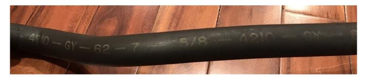
Again, If we are assuming the date code is 62-7 (July 1962?) it still could be correct, but the hose would've been over a year old. Still, given that Factory A/C was a low production option, it may be possible that these parts sat around that long. Anyway, it's what I pulled off the car, so I assume it was correct.
