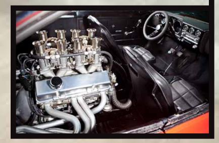
Headphones are available for those rides when hearing preservation takes precedence over the din of a barely muffled Chevy V-8. Only two things keep the whirring water-pump pulley from biting the occupants' elbows: the flush bolts that Siano installed in place of hex-head screws and every human's natural preservation instincts.
