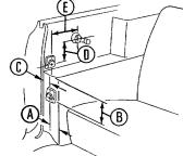
2) DRILL TWO (2) 1/8" HOLES AND SECURE RETAINER TO BODY.
