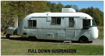
Air Ride e-3 fully automatic self-leveling air suspension. Wilwood power 12.2" disk brakes on front. Power rear drum brakes on separate hydraulic circuit. Upgraded steel front suspension and steering assembly. Upgraded rear suspension. 225/60-15 Fusion tires on front on HD Cragar steel truck rims. 245/45-17 XL Kumho tires on rear on HD Cragar truck rims.
