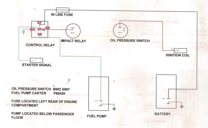
30 to 87a normally closed 30 to 87 normally open 85 coil ground 86 coil actuate relay is diode protected
